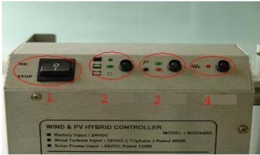
1、 Switch to be “ON” position ,wind generator is working condition. Switch to be “STOP” position, wind generator to be stop position.
